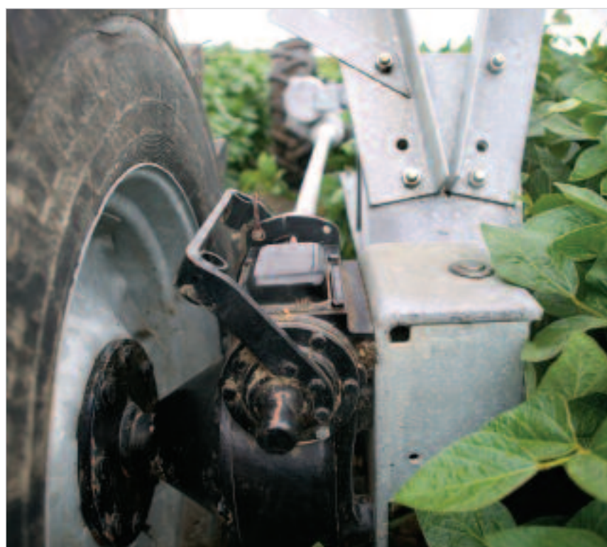
Zimmatic's tow/non-tow final-drive gearbox uses a bale engagement lever to disengage the gearbox for towing. When you're ready to irrigate, simply re-engage the gearbox with the lever.
